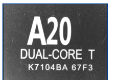
环氧树脂填充打标效果 Marking Effect of Epoxy Resin Filling
