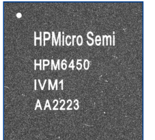
环氧树脂单线条打标效果 Marking Effect of Epoxy Resin Single Line
